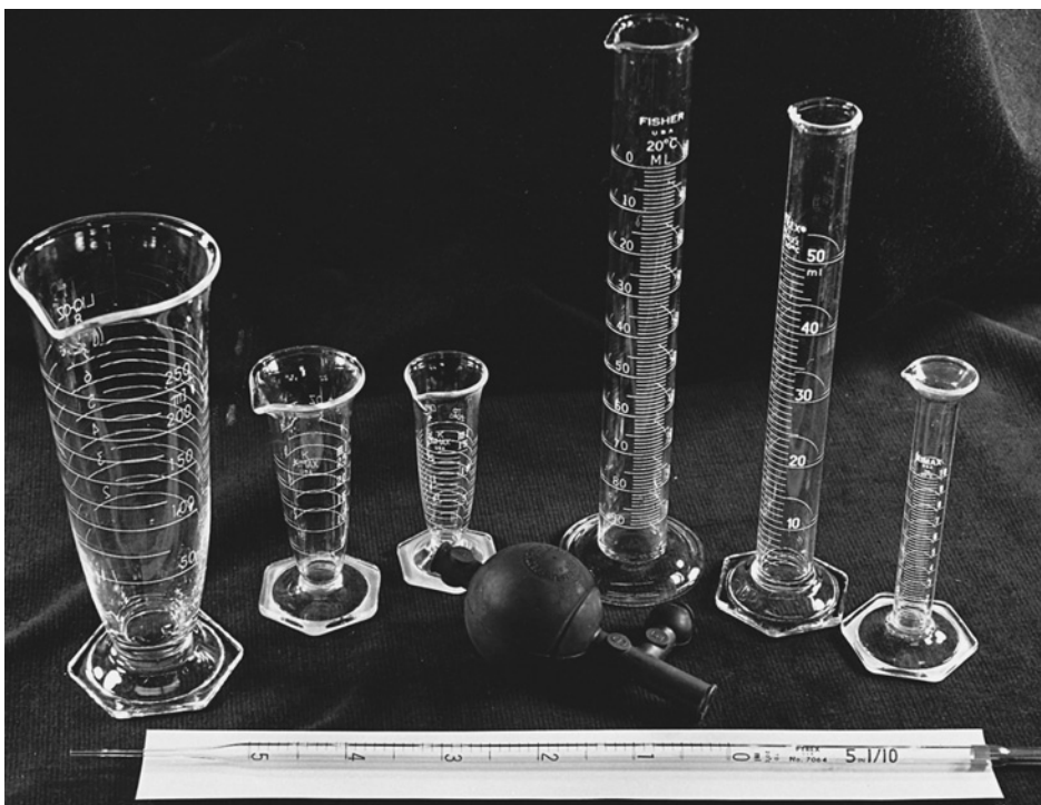
FIGURE 3.1 Examples of conical and cylindrical graduates, a pipet, and a pipet-filling bulb for volumetric measurement.
