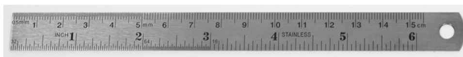
FIGURE 2.3 Ruler calibrated in millimeter, centimeter, and inch units. (Courtesy of Schlenker Enterprise, Ltd.)
