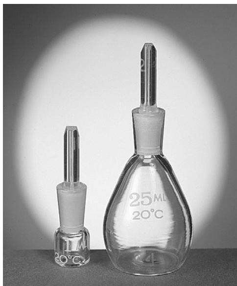
FIGURE 5.2 Examples of pycnometers used to determine the specific gravity of liquids. Shown are 1-mL and 25-mL sizes. See text for description of their use. (Courtesy of Thomas Scientific.)
